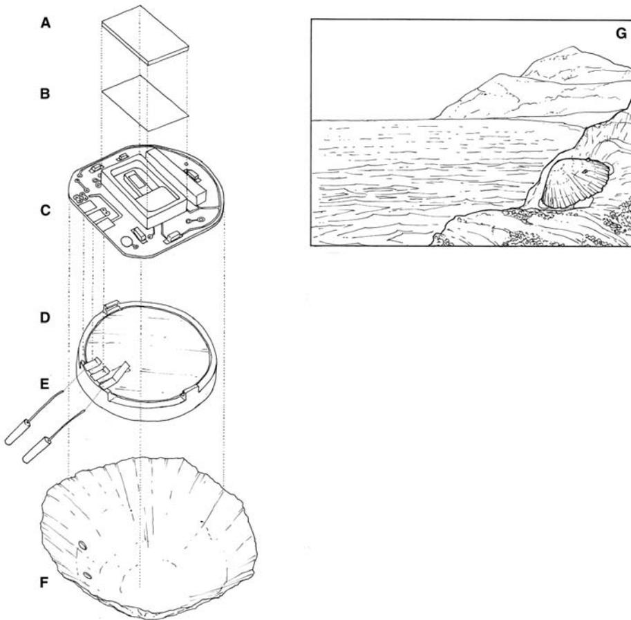
Fig. 7. Humidity logger mimicking a *Patella* sp. A: viscose pad, B: Tyvek polyethylene fiber paper, C: DS1923 iButton circuit board, D: DS1923 iButton battery, E: constantan wires (larger diameter) connected to wirewrap wires. F: *Patella* sp. shell with two holes to allow the constantan wires to protrude, G: Representation of a humidity sensor deployed in a rocky shore during low tide.
