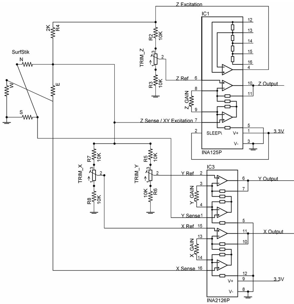
Fig. 11. Schematic Diagram of force sensor circuit. On the left hand side of the circuit is the CTS "SurfStik", with strain gauge resistors on the four sides (N,S,E,W) of the ceramic post.
