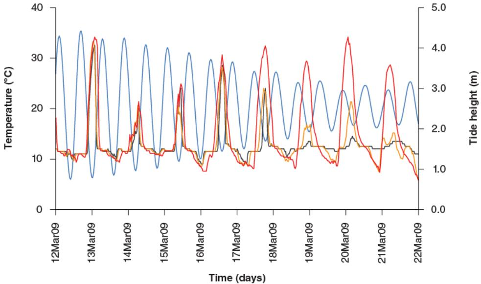
Fig. 6. Example of robolimpet data from an exposed rocky shore in Biarritz (SW France) taken between March 12<sup>th</sup> 2009 and March 22<sup>nd</sup> 2009. Times are in GMT. The black, orange and red lines show temperatures as measured by low-, mid- and high-intertidal loggers. Tidal heights are shown by the blue line.
