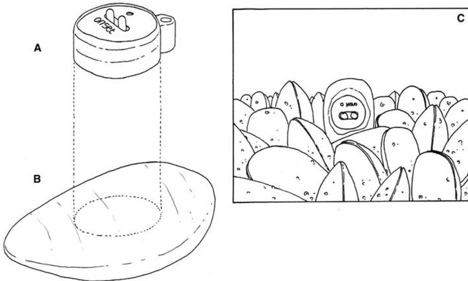
Fig. 1. Temperature logger mimicking a *Mytilus californianus* (robomussel). A: Onset TidbiT logger, B: Evercoat Everfix epoxy cast of a *M. californianus*, C: representation of a robomussel deployed in a mussel bed in the field.
