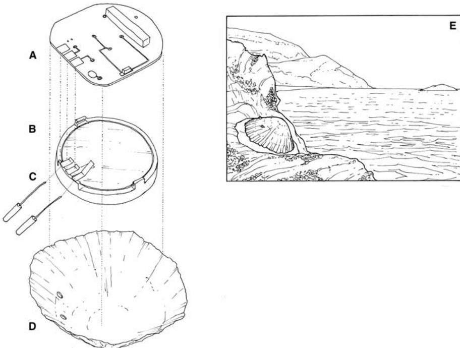
Fig. 4. Exploded view of the different parts used for building a temperature logger mimicking a *Patella* sp. (robolimpet). A: DS1922L iButton circuit board, B: DS1922L iButton battery, C: constantan wires (larger diameter) connected to wirewrap wires, D: *Patella* sp. shell with two holes to allow the constantan wires to protrude, E: representation of a robolimpet deployed in a rocky shore during low tide.
