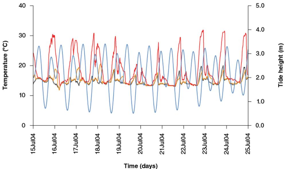
Fig. 3. Example of robomussel data from an exposed rocky shore in Seppings Island (SW Canada) taken between July 15<sup>th</sup> 2004 and July 25<sup>nd</sup> 2004. Times are in GMT. The black, orange and red lines show temperatures as measured by low-, mid- and high-intertidal loggers. Tidal heights are shown by the blue line.
