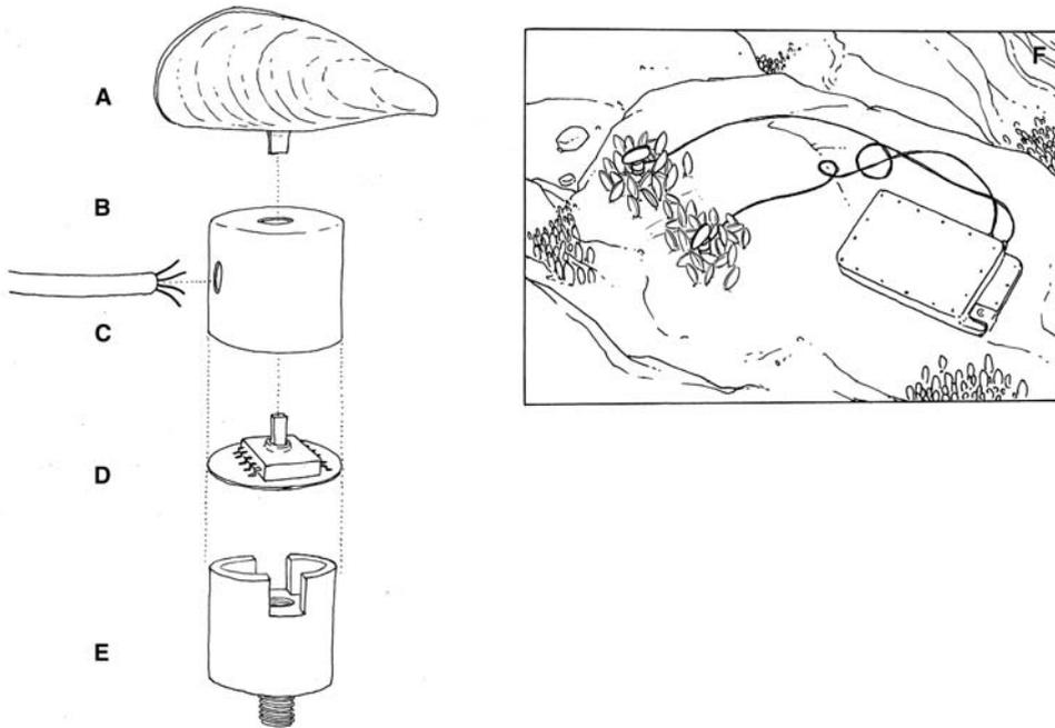
Fig. 10. Wave force logger mimicking a *Mytilus edulis*. A: polyester mussel model, B: copper pipe cap, C: sensor cable, D: printed circuit board with "SurfStick" sensor, E: polycarbonate plug with threaded rod for attachment. F: two wave force loggers deployed in musselbeds in the rocky intertidal together with an aluminum housing protecting the data logger.
